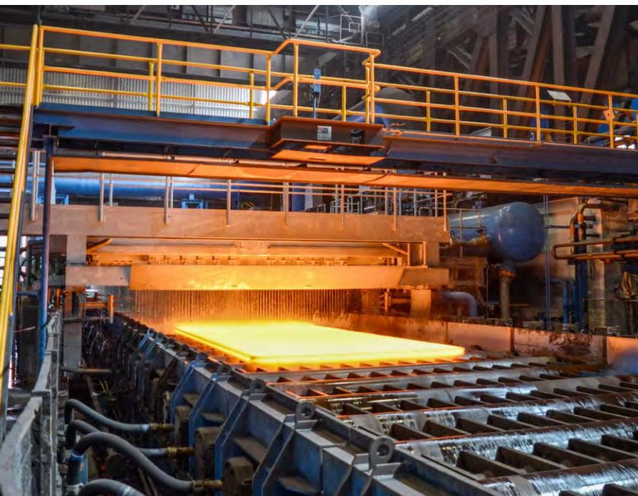
**49 Production of TMCP steel plates up to 100 mm**
